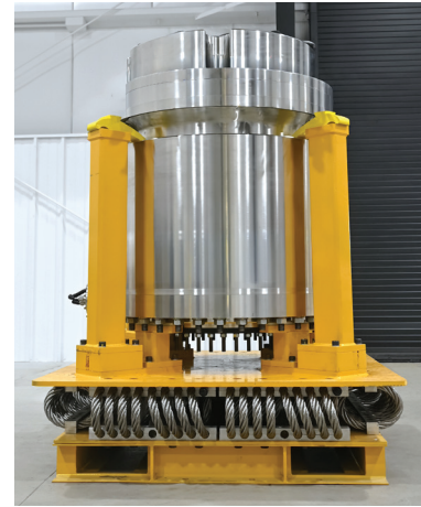
NTP Engineering Development Unit (EDU) designed, built and delivered to Marshall Space Flight Center for cold flow testing
