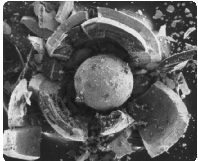
A scanning electron micrograph of a coated nuclear fuel particle after a crush test
