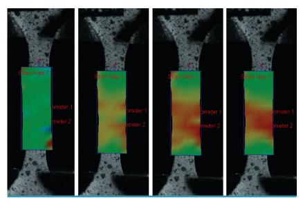
Strain mapping using DIC system
