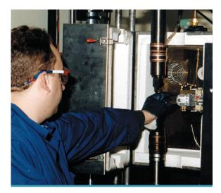
Elevated temperature tensile testing
