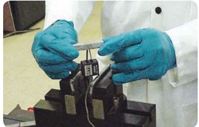
Three-point bend testing
