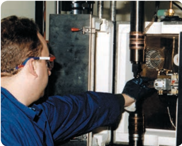
Elevated temperature tensile testing
