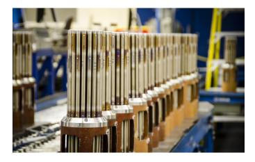
Every aspect of each fuel bundle, from the zirconium tubes and natural uranium pellets, to the welds and spacing between tubes, must meet stringent quality criteria.
