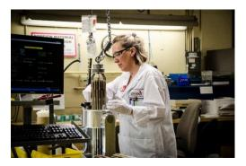
At the Peterborough facility, fuel manufacturing operations involve the loading of fuel pellets into Zircaloy tubes, sealing, and welding of the tubes to produce fuel elements and the assembly of the fuel elements into fuel bundles. The basic assembly process is described in Figure 4.
