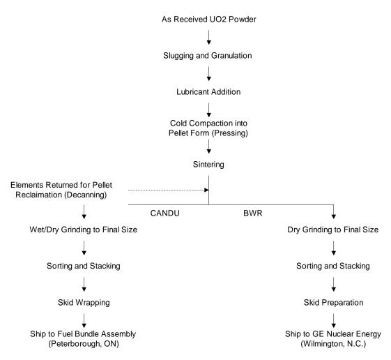
Figure 2: Uranium Fuel Pellet Manufacturing Process
