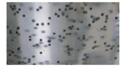
During TRISO production, spherical particles are hydraulically transported from the forming column to the collection vessels.
