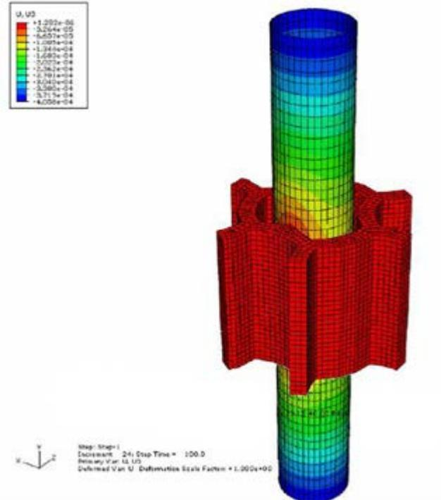
Abacus FE model of tube and tube support interaction
