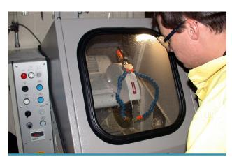
Precision abrasive cut-off saw
