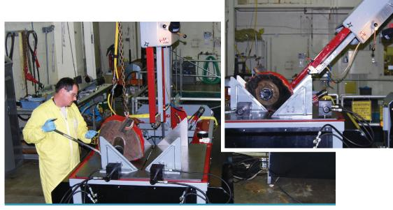
Sectioning control rod drive mechanism nozzle and surrounding reactor vessel head material on large capacity vertical band saw. Blade angle range is ±45° (inset)
