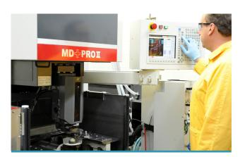
CNC electrical discharge milling machine
