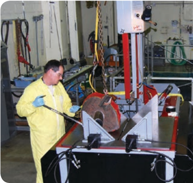
Sectioning Control Rod Drive Mechanism (CRDM) nozzle and surrounding reactor vessel head material on large capacity vertical band saw. Blade angle range is \pm 45^\circ (inset)
