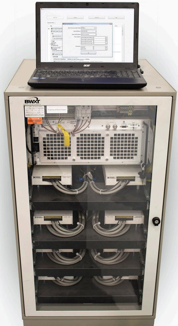
ASTE/d's field data logging function supports high-frequency sampling and recording of a large volume of analog and digital field I/O signals. Using this function, the field I/O signals of an in-service I&C system can be connected to ASTE/d, and data logging can proceed non-intrusively and unattended during normal system operation. Engineers can leverage an extensive suite of offline examination and analysis tools developed by BWXT to evaluate the vast amount of recorded data.
