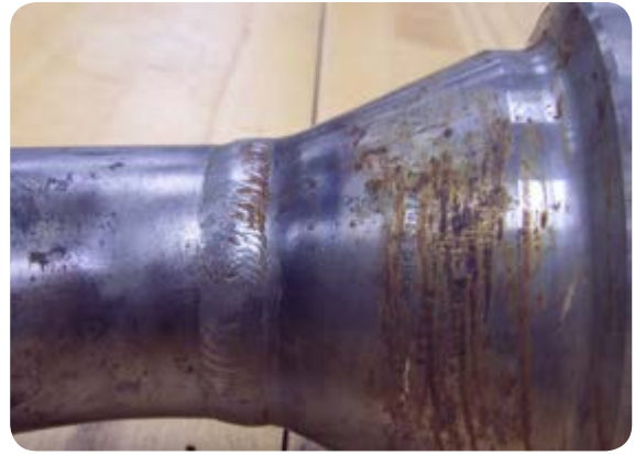
CANDU feeder tube Grayloc weld region
