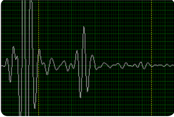
A-scan from tube adjacent to Grayloc weld
