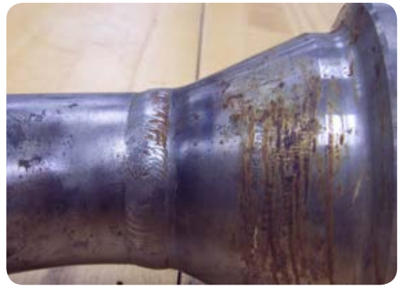
CANDU feeder tube Grayloc weld region
