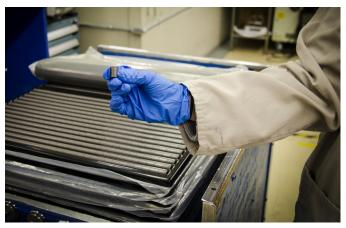
BWXT NEC's Toronto facility produces the natural uranium ceramic pellets needed for CANDU® fuel bundles.
