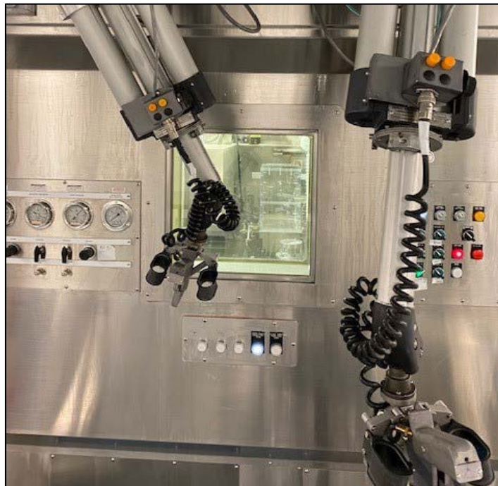
Figure 2: A hot cell at BWXT Medical
