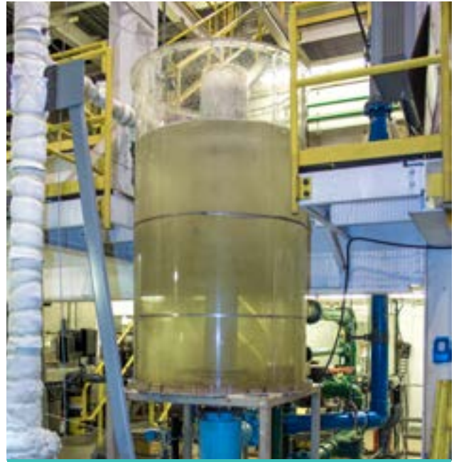
BWXT offers dynamic flow visualization for experimental testing through use of an air / water flow loop and high pressure borescopes.
