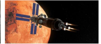
We are working with NASA on its nuclear thermal propulsion (NTP) project in hopes of powering a future crewed mission to Mars. Compared to traditional chemical propulsion, NTP's high-energy density and improved spacecraft thrust can shorten interplanetary travel times by up to 50% and improve crew safety by reducing exposure to cosmic radiation. We are also helping NASA reduce the development time and costs of a mission to Mars.
